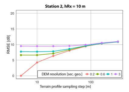
The above results show a strong correlation between DEM parametrization and final outcomes of the Recommendation ITU-R P.1546-5 models. Each time when the spatial resolution of the digital map is lower and profile sampling step is higher the RMSE is rising. For instance, the coverage of station 1 for DAB+ mobile reception/95% location for parameter {3"/320 m} is about 50% higher than for {0.2"/5m}. The coverage visualization matrix is presented in Figure 5.
